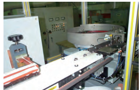
Figure 3 Vibratory Bowl Feeding Arrangement into Induction Coil 图三 震动盆送料处理进入感应线圈处
