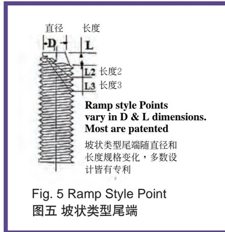
The second class consists of a formed shape on the end of the bolt. The one most commonly seen is ramp-like in appearance and there are several patented variations being currently offered for sale (Fig. 5).
