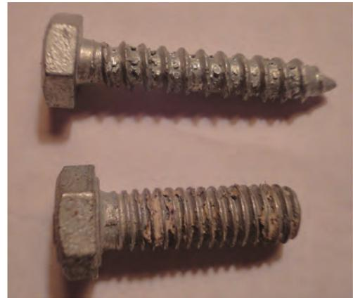
Fig. 3 Screw Threads with Zinc Clogs
