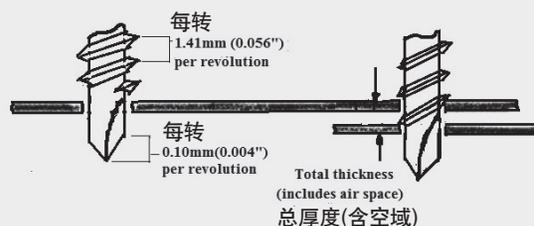
Drilling Stackup-M4.2 x 1.41 (#8-18) drill screw
