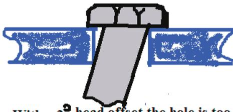
**With a 2° head offset the hole is too small for the bolt to pass through without interference at the underhead fillet**
