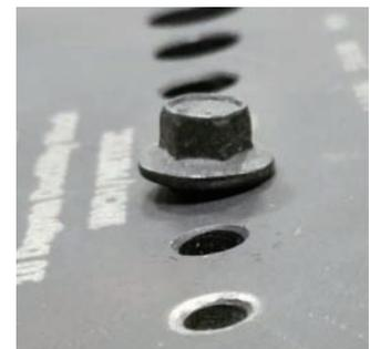
3. Strike the head of the screw with a hammer or other suitable device until it conforms to the angled surface. That is until the bearing surface of the head is flat against the angled surface. It may take more than one blow with a hammer to bend the screw head. (Fig.3 & 4)
