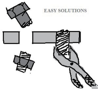
The worst case scenario is having to drill out the bolt fragment and enlarge the hole to the next larger size that will fit, if possible. Check for clearances and corollary damage to other components to insure assembly without undue interference.
