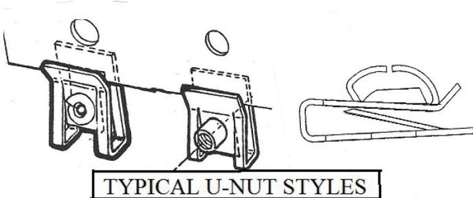
out from the backside will force the screw to cut new threads as it turns out. The sheet metal is softer than the screw and has probably stripped. If the backside is not reachable, use a vise grip type tool to work the screw out, prying as necessary. Replacement with the next larger size screw is required. The same solutions apply if the screw is jammed and does not turn. This works well if the screw head is large enough to afford a good grip.
