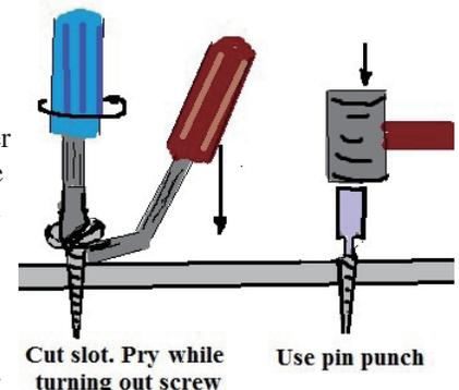
Cut slot. Pry while turning out screw Use pin punch
