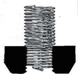
INSERT FOR STRIPPED THREAD REPAIR
