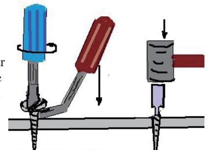
Cut slot. Pry while turning out screw      Use pin punch
