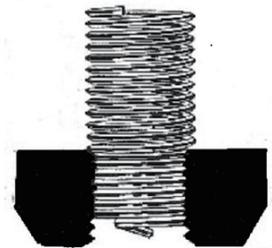
INSERT FOR STRIPPED THREAD REPAIR
