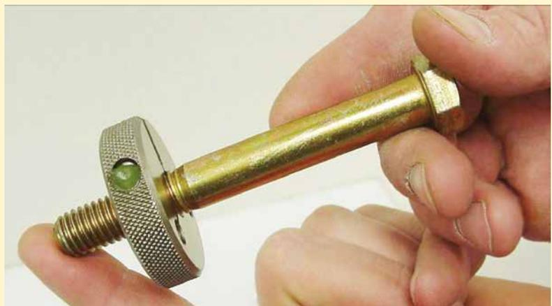
NoGo or Not Go thread ring gages have some not so straight forward rules. You would think that since the name of the gage is NoGo, that it should not even start to go onto the bolt threads. For practical reasons, this is not the case. Also, not all standards actually agree on how far the NoGo thread ring should be allowed to go onto a screw or bolt thread.
