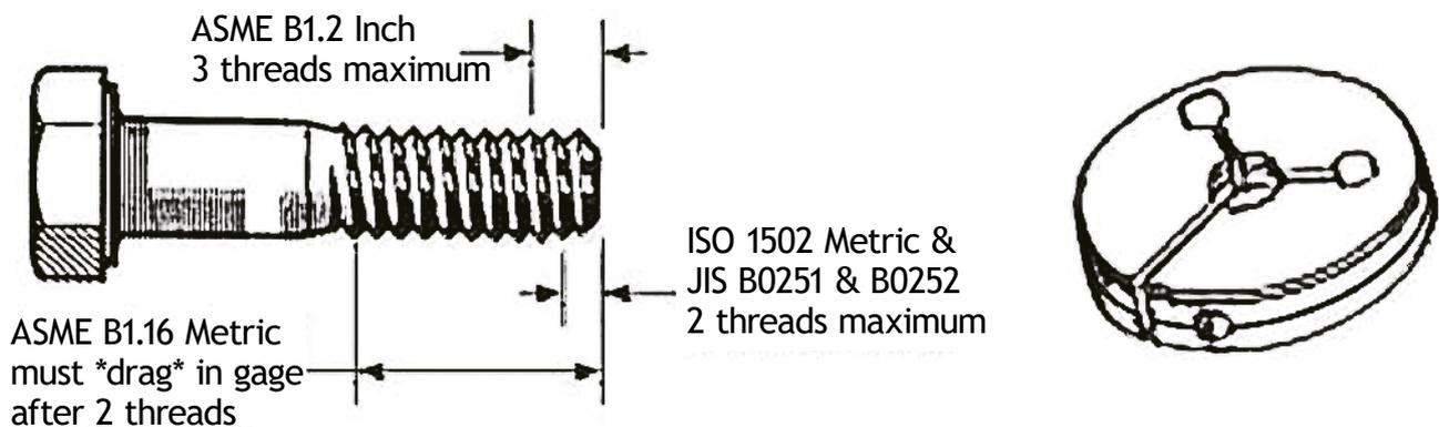
So the information we have from the standards referencing the rules for NoGo thread ring gages on external threads range from The NoGo ring stopping after 2 turns to allowing the Nogo thread ring gage to pass completely over all the threads only if a definite drag is felt. What are we to do with this information, and what happens when two gages provide different results?
