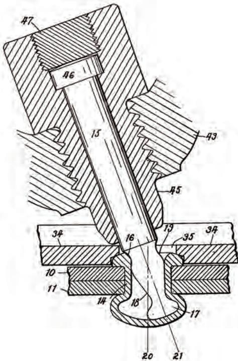
Figure 2. Deshon et. al. riveting device [US Patent 2,185,939]
