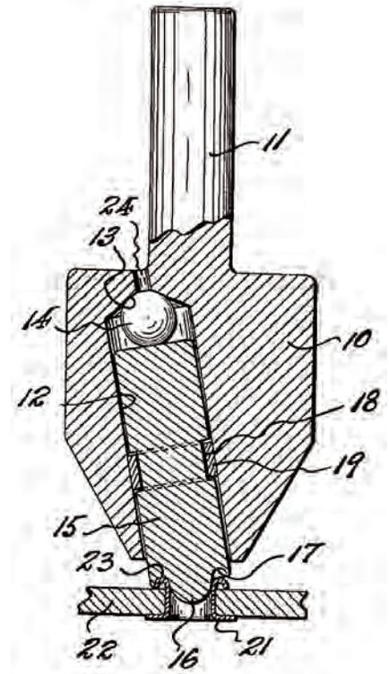
Figure 1. Bregen riveting tool [US Patent 2,739,726]
