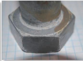
Fig. 5. Illustrating embedment of the ridges into the bolt head
