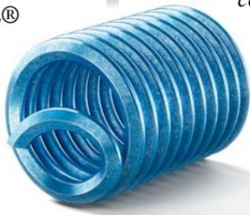
The HELICOIL® Smart thread insert, which is made from a wire with rhombic profile, is also formed into an elastic spiral. As to the Free Running version, thread by thread it is a completely free running coarse thread. The result is a true to gauge internal thread including the last thread which is in every case threadable. It produces high strength threads transferring forces from flank to flank into the holding thread.
