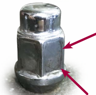
Fig. 4 Abused wheel nut having markings
