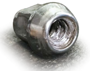
Fig. 5 Thread damage on the nut
